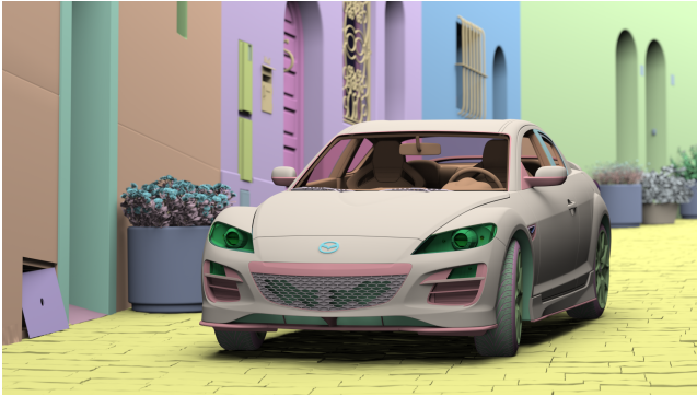
Figure 3: The material IDs assigned to the primitives of the Mazda scene, visualized with different colors. Our method sorts the ray hits by material ID before shading, which is enough to achieve high SIMD utilization.
