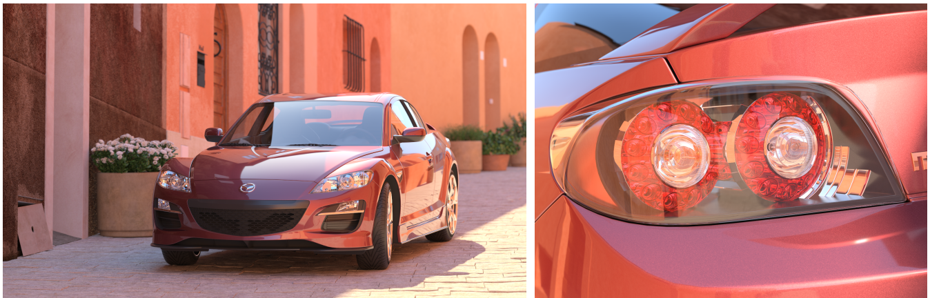
Figure 1: The Mazda scene (5.7M triangles, 76 materials) path traced using our stream-based shading coherence extraction method. For this scene, our coherent shading algorithm achieves 90% utilization of 8-wide SIMD and reduces the shading time by 2× compared to simple 8-wide packet shading. This results in a total speedup of 35%. For scenes with more complex shading, we have measured speedups up to 3×.
