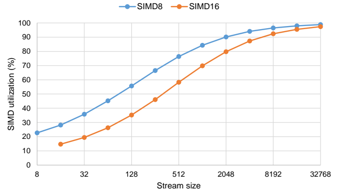
Figure 10: 8-wide and 16-wide SIMD utilization for shading the Mazda scene using our method (without path regeneration). With 2048 rays per stream, doubling the SIMD width causes only 10% reduction in SIMD utilization.
